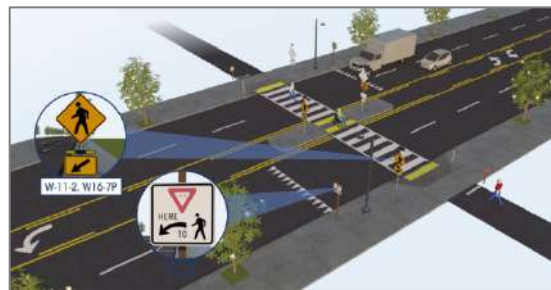
Figure 6: RRFB Example, Federal Highway Administration
