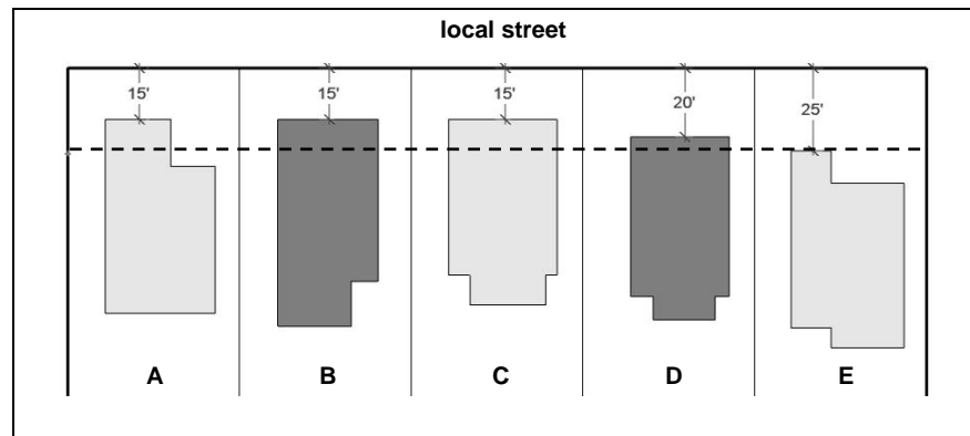
Illustration 4.1: Contextual Front Setbacks. (The required front district setback in the illustration is 25 feet, shown by the dotted line. There are existing houses on sites A, C, and E. A house built on site B may have a front setback of just 15 feet, which is the average of the front setbacks of the two abutting lots. A house built on site D may have a front setback of 20 feet, which is half-way between the front setback on the abutting lot that is lower than the district requirement (lot C) and the required front setback.)
