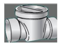
A backwater valve is a prevention device used to prevent outbound water flowing through a dwelling's drain pipes from re-entering, or "back-flowing", into a home. A backwater valve contains an automated gate that senses a reverse flow in the pipe and completely closes the line. When the water stops coming towards the home, the gate will open back up and allow flow to resume. A backwater valve must be installed by a licensed plumber at the homeowner's expense.
