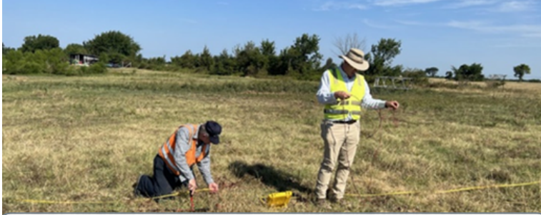
Environmental Engineering Division, Utilities Department and HDR Engineering Conducting Four Pin Field Testing on the OOWA Waterline Investigation Testing the Soils for Resistivity.
