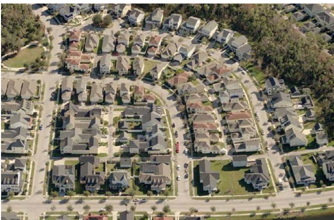
Interconnected street network is encouraged
