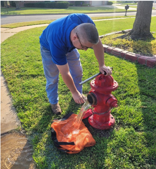
Justin Mitts testing water for chlorine residual.
